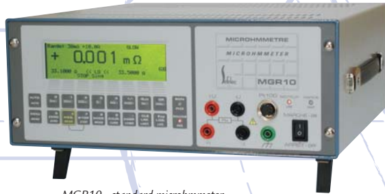
MGR10 - standard microhmeter MGR10A - mains or battery version MGR10B - contact resistance version MGR10C - pyrotechnic version
